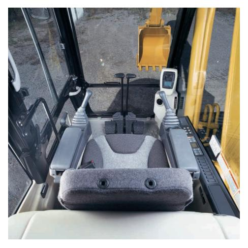
**Operator Environment.** The 312C operator work station is quiet with ergonomic control placement and convenient adjustments, low lever and pedal effort, ergonomic seat design and highly efficient ventilation.
