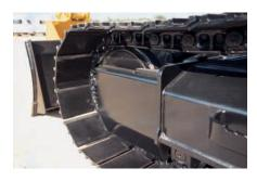
**Idler Guard.** An idler guard, which is integral to the track roller frame is standard. This guard helps maintain track alignment while traveling or working on slopes.
