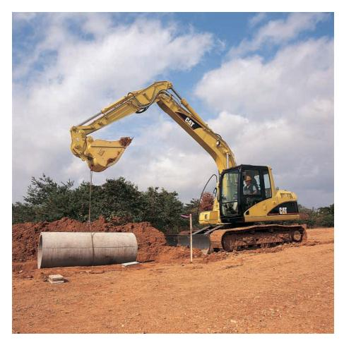
**Bucket Linkage.** The bucket linkage on the 312C includes the bucket cylinder, idler link and power links.
