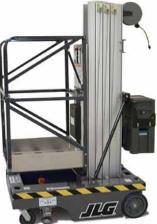
They can be loaded in a standard truck bed or lifted, using the six-inch wide fork pockets, making them easier to transport. The anodized mast gives you more stability and less deflection and sway. The mast-guide system doesn't require lubrication for the life of the machine.
