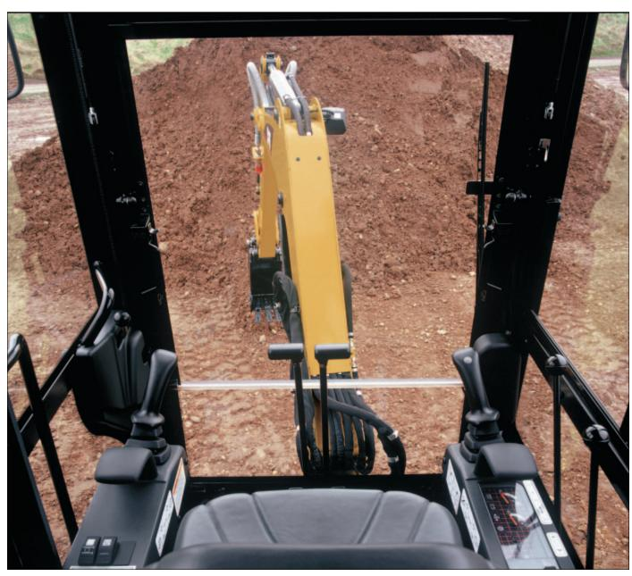
**Excellent viewing** to the work tool is possible with large windows and offset swing post. The curved hood and large rear glass give superior viewing to the rear. The easy-to-open front window and sliding right-side window offer excellent ventilation.
