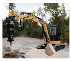
**Auxiliary Lines and Connectors.** The auxiliary lines and connectors including quick connections are fitted as standard, meaning the Cat 303C CR come ready to work. Hammer (one-way) and auger (two-way) auxiliary lines are also fitted as standard.
