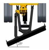
**Angle Blade Positioning.** The angle blade can be positioned straight ahead or angled up to 25 degrees to the left or right reducing the number of times required to back-up and reposition when backfilling thus reducing operation time.
