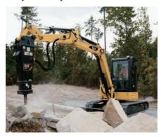
Auxiliary Lines and Connectors. The auxiliary lines and connectors including quick connections are fitted as standard, meaning the Cat 305C CR comes ready to work. Hammer (one-way) and auger (two-way) auxiliary lines are also fitted as standard.
