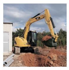
**Compact Radius Design.** The 308C CR is a compact radius version of the 307C. It is designed to work in a 2850 mm (9 ft 8 in) wide area.
