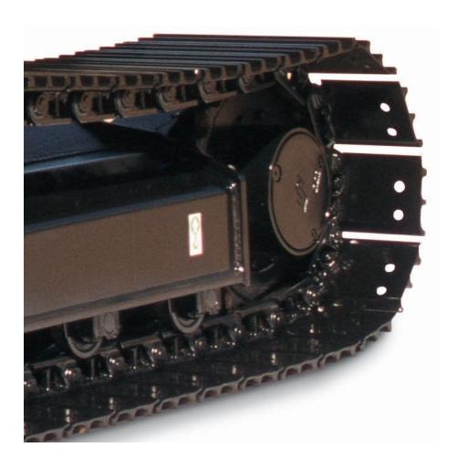
**Undercarriage Design.** The 308C CR uses a standard undercarriage with the same basic design as the 307C, ensuring high reliability.
