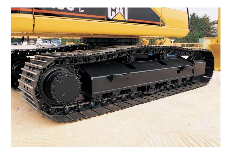
**Structures.** The 315C structural components and undercarriage are the backbone of the machine's durability.
