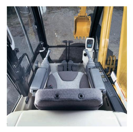
**Operator Environment.** The 315C operator work station is quiet with ergonomic control placement and convenient adjustments, low lever and pedal effort, ergonomic seat design and highly efficient ventilation.
