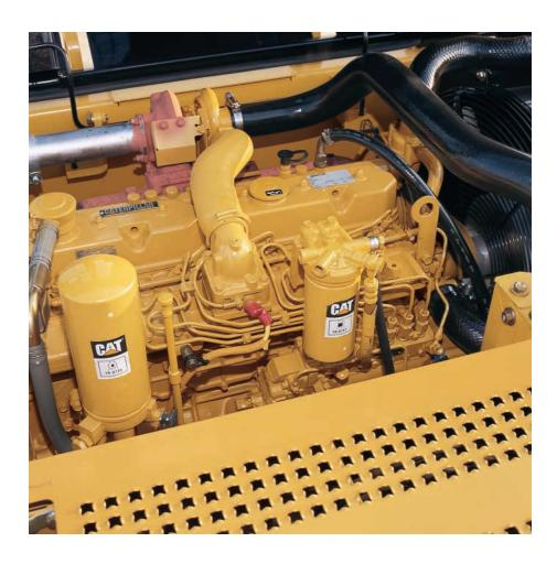
**Torque Rise.** The engine is designed for high torque rise at medium speeds — a feature that is especially beneficial for heavy-duty use.
