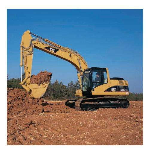
**Buckets.** To meet customer needs, five bucket sizes are available for heavy-duty applications. High tensile-strength steel is used in high-stress areas for excellent wear and shock resistance. The side and bottom wear plates and cutting edges are reinforced for extra protection.
