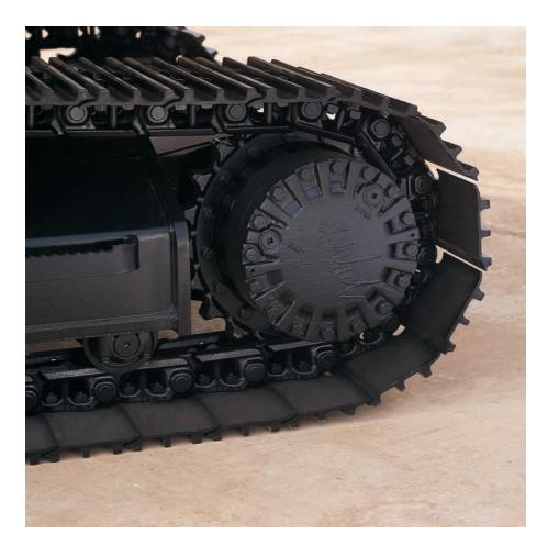
**Track Types.** The 318C is available with two different track types: long and long narrow.
