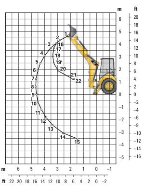
Lift Capacities are over-end values. Machine equipped with 4WD, OROPS, 0.96 m<sup>3</sup> (1.25 yd<sup>3</sup>) general purpose bucket, and 116 kg (255 lb) counterweight. Extendible stick includes 488 kg (1,075 lb) counterweight.
