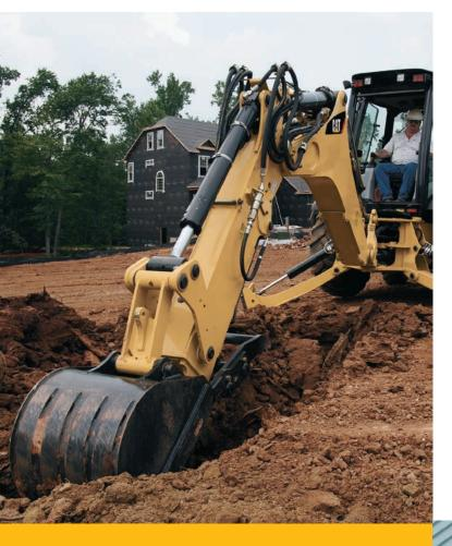
The 420E has a load-sensing, closed center hydraulic system, which closely matches power and flow to the demand needed by the implements. So whether you're in full trenching mode, or delicately digging around services, you are in control. In applications such as production trenching, speed is important and the system will match the flow needed to get the job done quickly and efficiently. The load-sensing hydraulic system also delivers:
