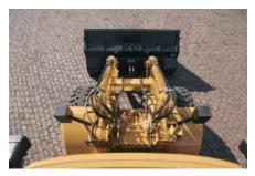
**8-Bar Linkage.** This linkage provides parallel lift to keep the load level throughout the lift cycle – particularly important when using forks. Parallel lift allows the operator to concentrate on placing the load, instead of retaining it. Visibility to the work tool is excellent.
