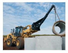
**Material Handling Arms.** Material Handling Arms move pipe, concrete blocks, highway dividers and other construction materials quickly and precisely. **Loader Rakes.** Loader Rakes are durable, high-capacity tools for land clearing and site clean up. Rakes are available with or without top clamps and in quick coupler and pin-on models.
