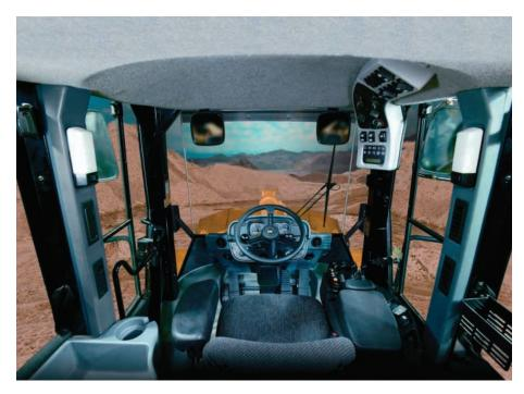
**CONTROLS.** The main control panel on the IT62H is located high on the right ROPS post – keeping everything within reach of the operator while maintaining visibility to the ground. Keeping all switches and controls conveniently placed allows better efficiency and improved productivity all while minimizing operator fatigue. The front dash panel is conveniently laid out for easy monitoring of gauges and operation of controls.
