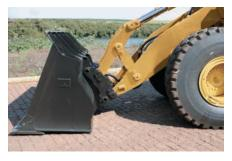
**Material Handling Buckets.** The material handling bucket is a flat-floor bucket used for handling stockpiled materials such as aggregates or other easy-to-load materials requiring moderate breakout force.
