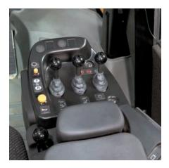
**Electrohydraulic Implement Controls.** Electrohydraulic implement controls on the IT62H provide the operator with incab programmable kickouts to prevent material spillage – improving productivity. The implement control console features an optional Forward/Neutral/Reverse switch allowing fast, easy directional changes to reduce cycle times.
