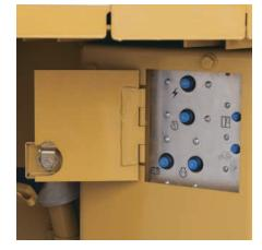
**ELECTRIC SERVICE CENTER.** Batteries, relay panel and an optional tool box are conveniently located below the left-side access platform. The engine shutdown switch is housed with the relay panel. A compartment integrated into the access platform contains the hood tilt actuation switch, master switch and jump-start receptacle.
