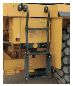
**ENTRY AND EXIT.** An open ladder design keeps debris build-up on the steps to a minimum. The ladder is at a  $5^{\circ}$  forward incline for easy entry and exit.
