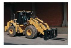
**Forks.** From pallet forks up through specialized logging arrangements, loader forks are available for a wide range of jobs.
