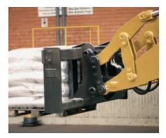
**Pallet Forks.** When used with a quick coupler, pallet forks increase the versatility of the machine; ideal for handling a variety of materials.
