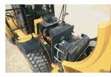
**ENGINE COMPARTMENT ACCESS.** The non-metallic hood on the IT62H has been redesigned and restyled from previous models. Side and top panels are stronger due to more robust reinforcement ribs – the change in contour also adds to rigidity of the hood.
