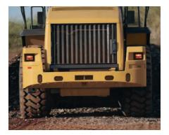
**Counterweight.** The one-piece counterweight is integrated into the IT62H design and styling. This 4389 lb (1991 kg) counterweight incorporates the rear lights into the top of the structure.
