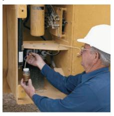
**S•O•S SERVICES.** Sampling valves on the IT62H allow quick access to engine, transmission and hydraulic oils for S•O•S analysis. Oil change intervals and other services can be optimized according to your work schedule, reducing downtime and managing expenses.
