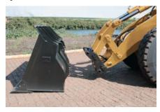
**Quick Couplers.** Quick couplers provide unmatched versatility for wheel loaders. The hydraulic model allows an operator to change attachments in seconds without leaving the cab. On the manual model, the operator must lock the pins.
