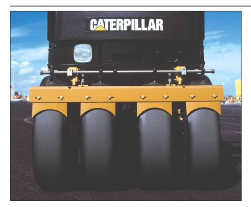
Steel front drum and rubber tires at the rear allow a single machine to function as both a double drum and pneumatic compactor.
