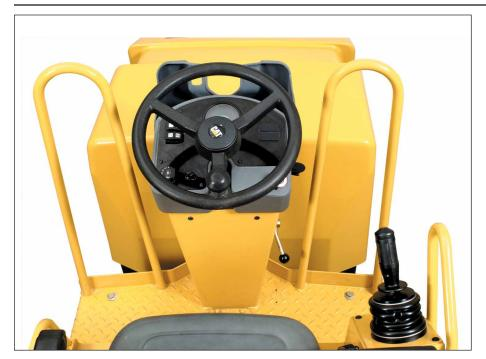
**Single propel lever control** provides simplified operation, making the machines a perfect fit for new operators.
