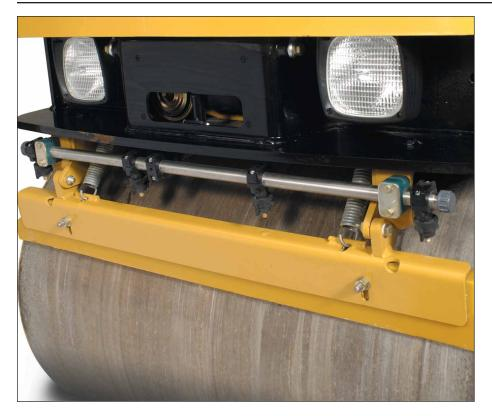
**Constant or intermittent spray capabilities** provide extended operation between refills.
