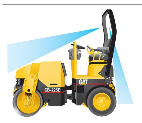
**Excellent forward visibility** allows the operator to see objects 0.58 m (1.9') high and 1 m (3.3') in front of the machine.
