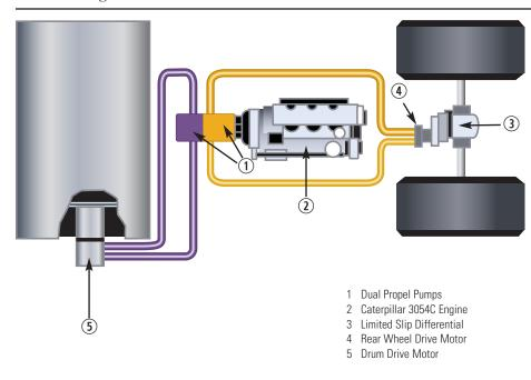
**Dual propel pumps** provide separate, balanced hydraulic flow to the rear wheel axle and the drum drive motors. Provides high gradeability and increases tractive effort in loose or poor underfoot conditions.
