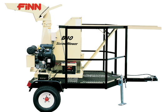
B40 Straw Blower Trailer Mounted (B40T)
