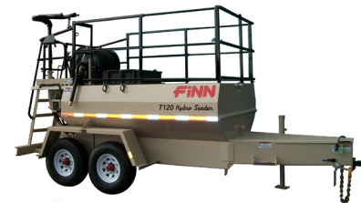
T120 HydroSeeder Straight Pull Trailer. (T120T)
