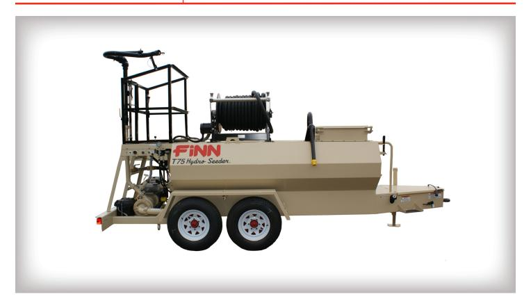
The FINN T75T HydroSeeder is the ideal 700 gallon tank working capacity for landscapers and contractors who need high powered performance and productivity. The T75T fits in the FINN line as the feature-filled package right between the small tank sizes and larger trailer-mounted models. Weighing in as a trailer unit with a fully loaded weight of 10,000 GVW, the FINN T75T satisfies the ideal towing requirements of a ¾ ton or a 1 ton truck without a commercial license.
