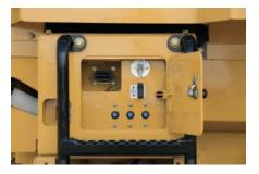
Electric Service Center. A lockable compartment located just below the left side access platform contains key electrical components such as the remote jump-start receptacle, battery disconnect switch, circuit breakers and hood actuation switch. The maintenance free batteries are conveniently located under the electric service center.
