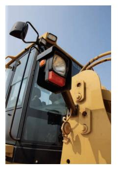
Lighting Packages. In addition to the standard roading lights, optional lighting packages are available for lowlight applications. Optional auxiliary halogen or High Intensity Discharge (HID) cab lights provide exceptional lighting for night work. A rotating beacon is available as a safety feature.
