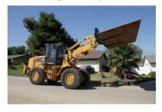
Load Sensing Hydraulics. The IT38H features a load sensing hydraulic system that supplies flow and pressure for the implements only upon demand, and only in the amounts necessary to perform the needed work thus providing a more efficient loader.
