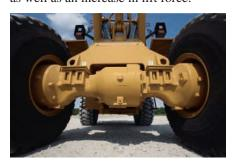
**New! Differential Lock.** Maximize productivity with the new hydraulic locking front differential. This standard feature provides operators with the confidence to maneuver through poor underfoot conditions with 'on the fly' engagement.
