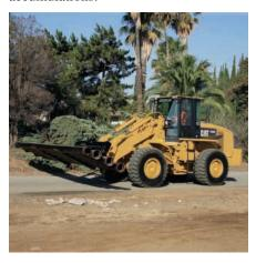
**Forks.** Logging, Millyard and Pallet Forks are available for forestry and material handling applications.
