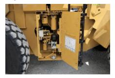
**Hydraulic Service Center.** Transmission and hydraulic oil filters are located in the Hydraulic Service Center, behind the hinged, right-side access ladder. The hydraulic oil tank can be drained from this location using the access port.
