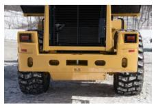
**Counterweight.** The one-piece counterweight is integrated into the IT38H design and provides added protection for the lights by incorporating them into the top of the structure.
