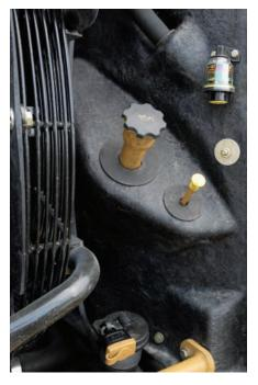
With the hood closed, quick checks of the engine oil level, coolant site gauge and air inlet indicator can be completed through the side service door.
