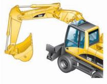
**Offset Boom.** The offset boom (5.2 m/17 ft 1 in) adds a major advantage and a high level of versatility to the machine, providing the ability to dig parallel to the machine's undercarriage. The combination with a tiltable ditch cleaning bucket increases machine versatility.
