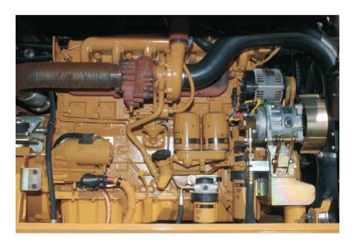
**Powerful Performance.** The 3056E DIT ATAAC engine delivers a net power of 103 kW (138 hp) at the rated speed of 2,000 rpm, and meets U.S. EPA Tier 2 emission standards.
