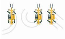
**Steering Modes.** The TH580B offers three steering modes (two wheel, crab and circle steer) to allow an operator to easily position the machine. Steering modes are selected by a single three-position rocker switch. Steering position sensors are fitted as standard to all steering modes to be changed while moving.
