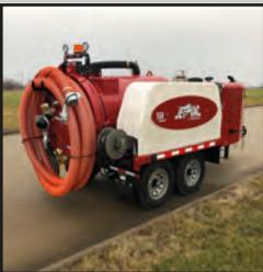
Streamlined water tanks provide you with 200-gallon of on-board water capacity, designed to keep the Center of Gravity low and well positioned over the axles to maximize tow-ability. Low water shutdown is standard to assist in eliminating the chance of running the water pump dry. Also Available are 2/165 gallon water tanks.
