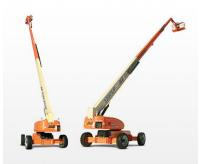
AN AVERAGE STRAIGHT TELESCOPIC BOOM MIGHT FEATURE A MAXIMUM PLATFORM HEIGHT OF 40 FEET, BUT IT'S NOT UNCOMMON TO SEE BOOMS OF 100 OR EVEN 200 FEET. Platform widths typically have a standard size of eight feet or larger, which is one of the widest bases compared to other aerial lifts. The stowed height of most telescopic booms is under 10 feet, and telescopic booms use diesel or dual fuel. Specialty Uses of Straight Telescopic Booms
